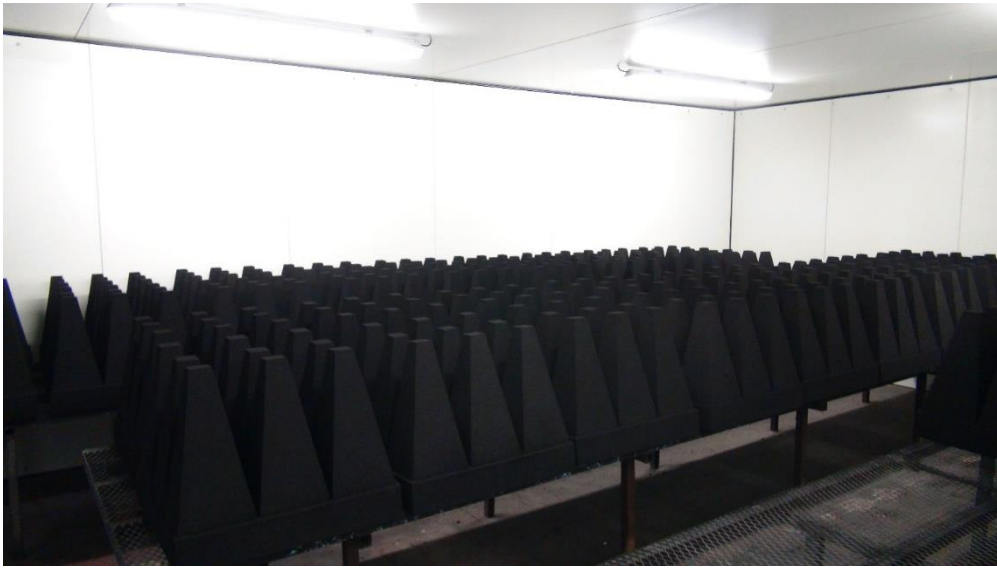
HPT Absorbers before painting
