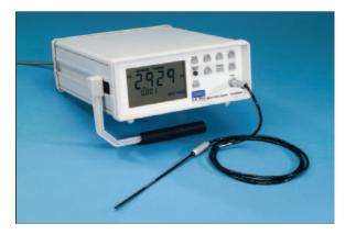
The Model 6010 Hall-effect Gauss/Tesla-Meter features F.W. Bell's exclusive Dynamic Probe Correction, along with temperature compensation and allows measurements up to 300 kG with a basic accuracy of 0.25%. Key features include Peak Hold, Max/Min Hold, Auto Zero, Auto Range, Relative Mode and Temperature measurement. The Model 6010 allows the user to select Gauss, Tesla or Ampere/Meter readings. The Model 6010 also features a corrected analog output (± 3 V Full Scale for each range),
