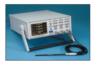
The F.W. Bell 7000 Series Gauss/Tesla-Meters lead the way for Advanced Hall Effect Magnetic measuring technology. The easy-to-use front-panel programming feature incorporates the latest in user control operations. The 7000 Series instruments are capable of simultaneously measuring and displaying seven different parameters per channel – 27 total parameters for the 7030 three-channel model.
